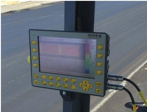
*The temperature profile is displayed along with the relevant GPS coordinates and weather data on the on-board computer and saved separately*
